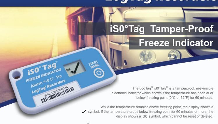
The iS0°Tag® can be used to monitor the temperature of any freeze-sensitive product such as vaccine, food, or specialty chemicals for up to 3 years. If a freezing event occurs the X symbol is displayed and the indicator is locked. Once locked, the indicator cannot be re-used.
