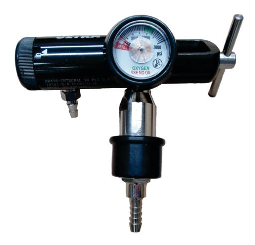
Dial Click Stop Constant Flow with pressure gauge to register cylinder pressure Oxygen delivery through Click-Stop Hand Dial Marked 0-25l/min Oxygen Cylinder Pressure Gauge Pressure Dial protected by a rubber ring Outer Body manufactured from Aluminium Inner Body Manufactured from Brass Minimum Input Operating Pressure 200 bars Output Pressure at Heyer: 3 - 6 Bar Male/Female Connection Included
