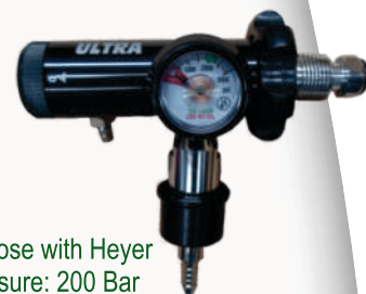
Ultra Pin Index with Heyer Inlet pressure: 200 Bar Outlet pressure: 3 - 6 Bar Increments: 1,2,4,6,8,10,12,15,18,20,25 \ell pm
