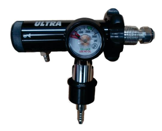
Dial Click Stop Constant Flow with pressure gauge to register cylinder pressure Oxygen delivery through Click-Stop Hand Dial Marked 0-25l/min Oxygen Cylinder Pressure Gauge Pressure Dial protected by a rubber ring Outer Body manufactured from Aluminium Inner Body Manufactured from Brass Minimum Input Operating Pressure 200 bars Output Pressure at Heyer: 3 - 6 Bar Male/Female Connection Included
