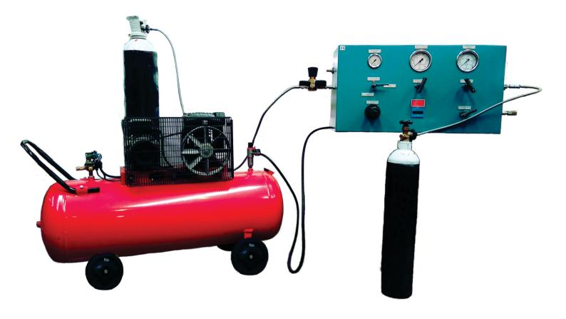
Portable 2-Stage Pneumatic (Air Driven) High Pressure Oxygen Refilling Booster system, including 200 litre Compressor with Purge Valve to release excessive high pressures.
