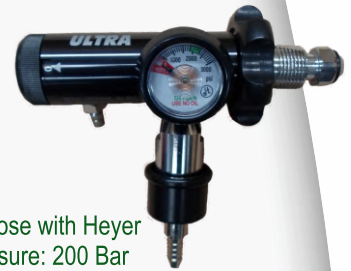
Ultra Pin Index with Heyer Inlet pressure: 200 Bar Outlet pressure: 3 - 6 Bar Increments: 1,2,4,6,8,10,12,15,18,20,25 \ell pm
