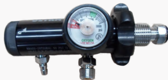
Ultra Bullnose with DISS Inlet pressure: 250 Bar Outlet pressure: 3 - 6 Bar Increments: 1,2,4,6,8,10,12,15,18,20,25 \ell pm
